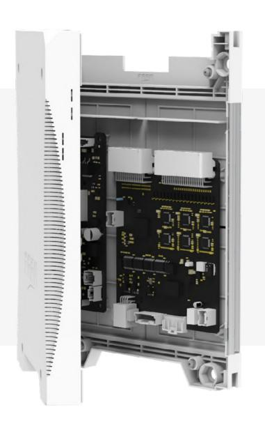
Protection levels as for both Cell Voltage and Cell Temperature (the most important ones as for lithium safety) are implemented. The first one by SW, the second one by pure HW. The latter acts as a further protection in case of failure of the SW one (uC failure).
